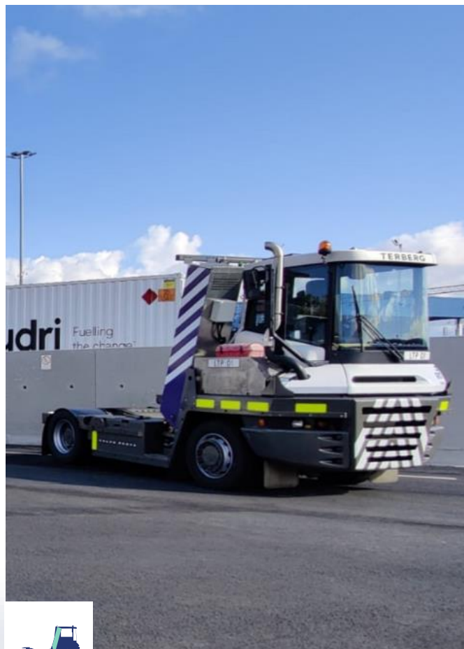
RORO TRACTOR TRANSPORT OF ROAD-TRAILERS BETWEEN SHIP AND TERMINAL
